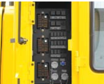
Compact fuse Box for Easy Inspection
