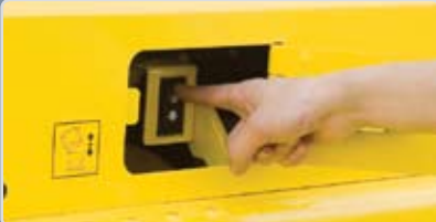
Cabin Tilting Automatic System Cabin tilting automatic system makes servicing of all power train components quick and easy. An electrically assisted hydraulic actuated cylinder tilts operator cabin to left side about 65 degrees for easy access to inside of truck components.
