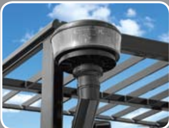
Visible pre-cleaner Efficient, accessible pre-cleaner provides for longer engine life.
