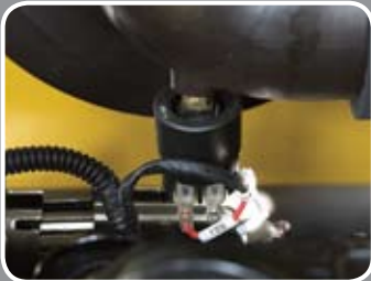
Electrically monitored air filter Air cleaner sensor alerts the operator of a restricted air filter and allows replacement before damage.
