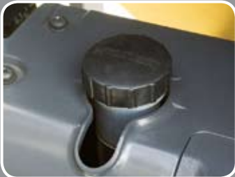
Brake fluid reservoir Highly visible, easily accessible reservoir makes for quicker daily inspections.
